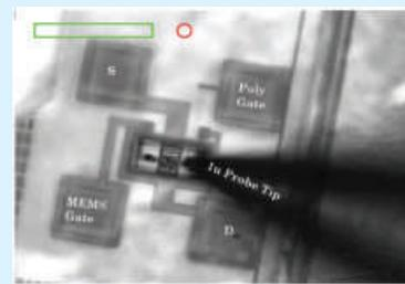
Suspended gate inertial sensor device
