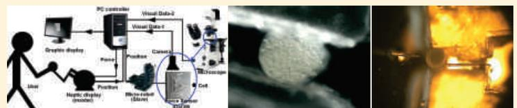
Figure 1. Bio-micromanipulation system comprising a haptic robot, miniature grippers, micro-positioners, and a microscope. A zebrafish egg-cell grasped and pierced is also shown.
