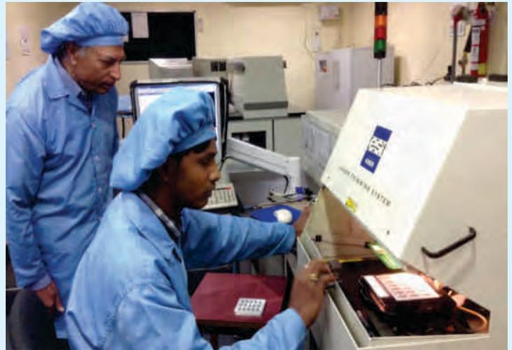
Active Laser trimming of Resistors
